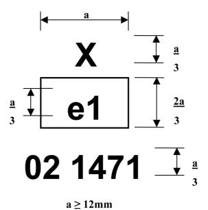
The device bearing the EC type-approval mark shown above is for a frontal protection system type-approved in Germany (e1) pursuant to this Regulation (02) under the base approval number 1471.
